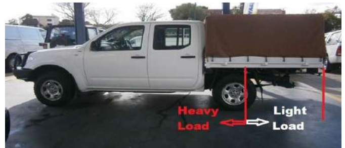
Incorrect length tray for the wheel base and load carrying capacity.
