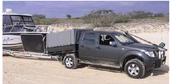
An extension hitch to a tow bar requires careful consideration to prevent this from happening.
